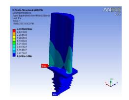
Figure 18: Stress Distribution in the Fir Tree Section of Material N 155
