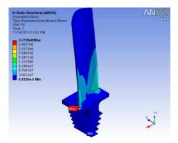
Figure 6: Von-Mises Stress of N 155
