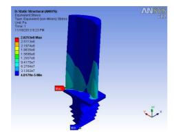
Figure 14: Stress Distribution in the Fir Tree Section of Material Mild Steel
