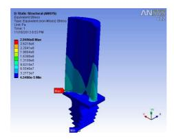
Figure 4: Von-Mises Stress of Mild Steel
