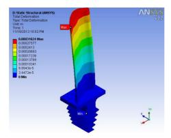
Figure 9: Deformation of N 155
