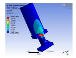
Figure 15: Stress Distribution in the I-Section of Material INCONEL 718
