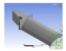
Figure 2: Solid Model of Turbine Blade with Fir-Tree Type Root
