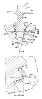
Figure 1: Fir Tree Type Blade Root
