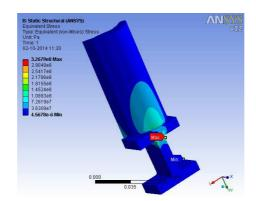
Figure 17: Stress Distribution in the I-Section of Material N 155
