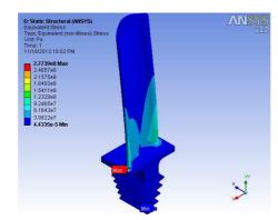
Figure 16: Stress Distribution in the Fir Tree Section of Material INCONEL 718
