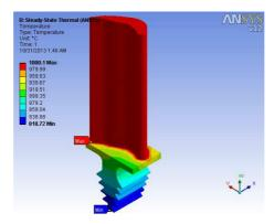
Figure 10: Temperature Distribution of Mild Steel
