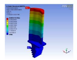
Figure 7: Deformation of Mild Steel
